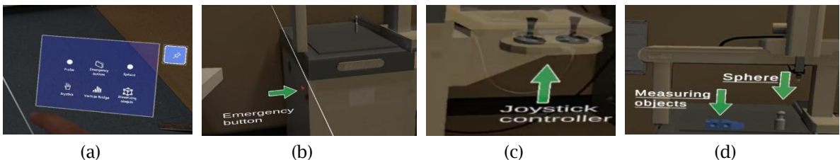
Fig. 6: CMM's component: (a) buttons, (b) emergency switch, (c) joystick, (d) object and sphere.
