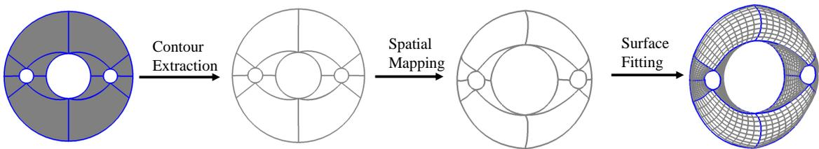
Fig. 5: Spatial spline surface generation process.
