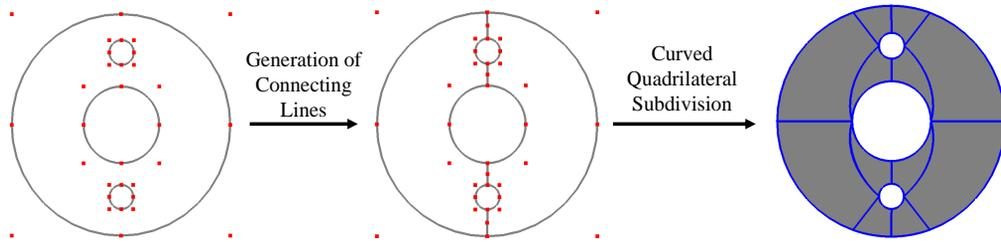
Fig. 4: Curved quadrilateral subdivision process.
