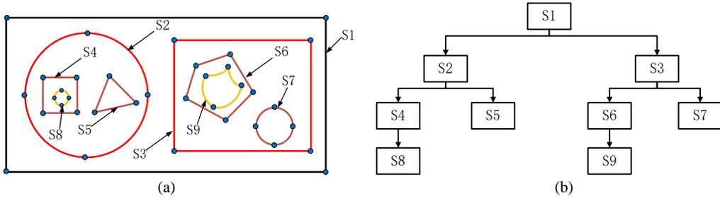
Fig. 2: Geometric domain inclusion tree.
