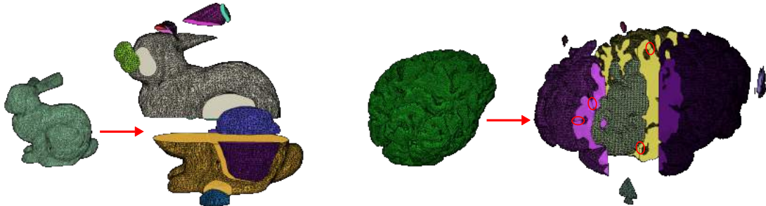
Fig. 2: Example of the cutting by plane operation for two different meshes, the results of which, at the right of each red arrow, are in topological view to observe the different volumes generated. On the right, Stanford bunny; on the left, a cerebral cortex, made up of several nested volumes (inclusion information are circled in red).
