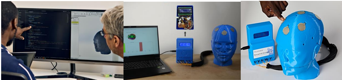
Fig. 4: (a) Back-end code, (b) Device GUI, (c) Pressure sensitive 3D printed head right.
