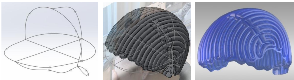
Fig. 2: Path for skeleton rigging (Left), application to cap (Mid), cap CAD model (Right).
