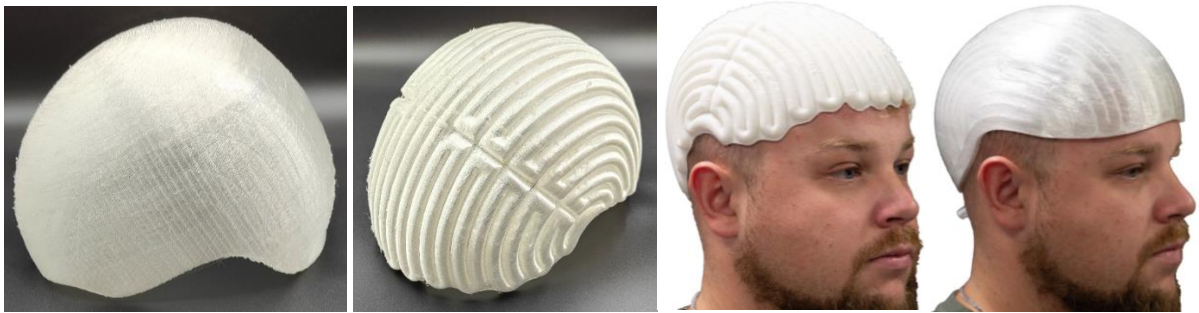
Fig. 5: 3D printed generic outer shell (left), standard printed cooling cap (left, mid), Customized cap (right mid), bespoke CAD customized cap (right).
