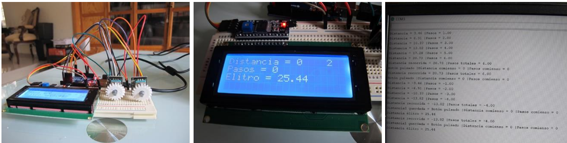
Fig. 1: Displayed on the LCD screen and the serial monitor distance traveled by the wheel.
