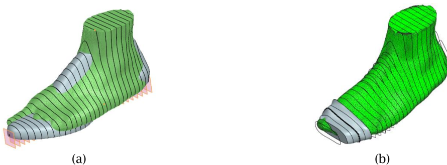
Fig. 5: An automatically constructed customized shoe last model: (a) Comparison of US9 wider foot (green) and US9 standard shoe-last (concrete); (b) An automatically constructed customized shoe-last model with wider forefoot region.
