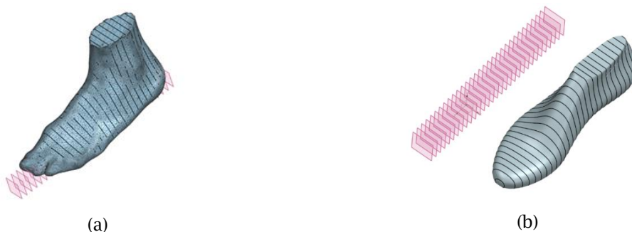
Fig. 3: N sections are intersected with the model to obtain the section curve diagram: (a) N sectional lines intersecting with the human foot model, (b) N sectional lines intersecting with the standard shoe last model.
