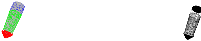
(a) Deposition head derived from risk-zone voxelization, distributed as 58%, 35%, and 7% of 13,820 voxels. Execution Time 0.024s. (b) Voxel model of 35,905 voxels obtained using the Open3D voxelization function. Execution Time 0.12s.
