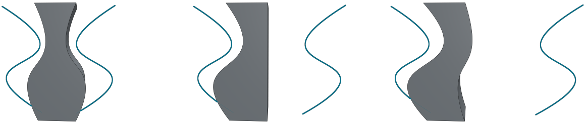
Fig. 5: Distance-based blending for multiple guide curves. First: Both curves are close, Second: Left curve is close, right curve is twice as far, Third: Left curve is close, right curve is 3-times as far.
