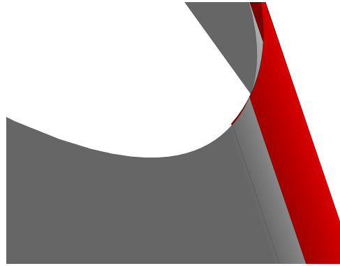
Figure 10: Recovery/Increase of TE radius from initial (grey) to updated (red)
